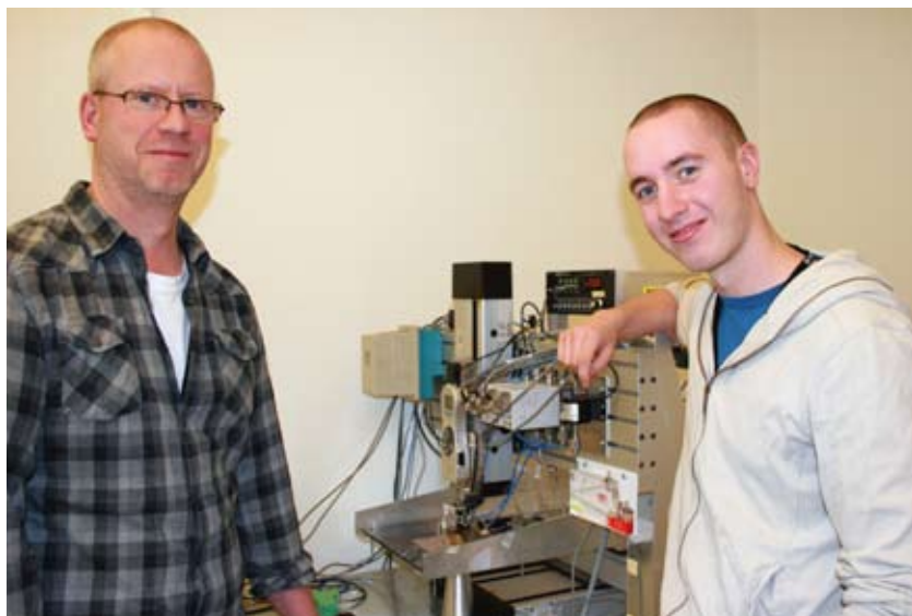
Mikael Bouveng and Alexander Waljanson demonstrating the Local Permeance Measurement Device. This unique equipment produces a map viewing variations in the permeability. The red areas indicate high permeance.
