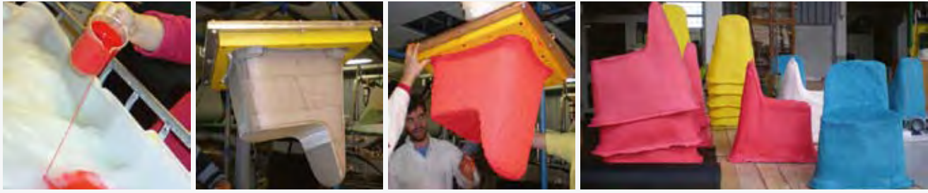
Pictures from the moulding process of the Södra Parupu chair in Markaryd, April 2009.
