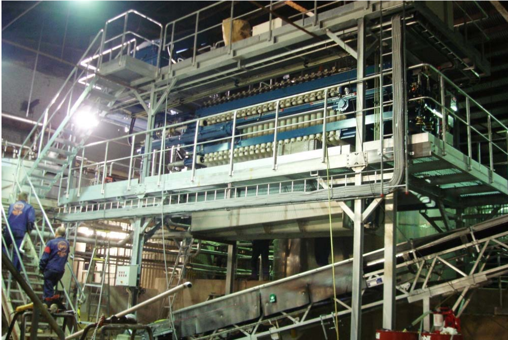
Figure 1. Interior view of the demonstration plant in Bäckhammar, showing the chamber filter press used for dewatering and washing of the lignin.
