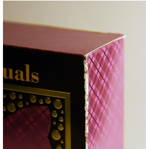
Crack in the color layer on the edge of the box
