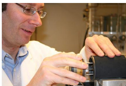
Insertion of a sample into the pyrolysis chamber.
